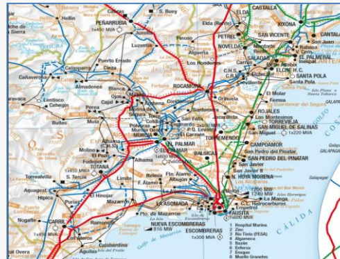
Murcia 220kV transmission path affected by N-2 outage
